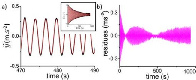
FIG. 4. (Color online) a) A few periods around 480 s: raw data (black dots) and damped sine fit (red line). Inset: full record. Agreement seem quite satisfactory. b) Residues from the fit showing a large and structured discrepancy between the data and the fitted curve.
