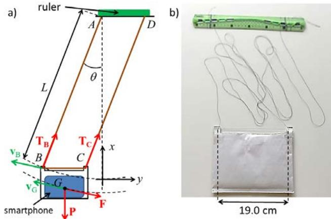
FIG. 1. (Color online) a) sketch and b) picture of our pendulum. The smartphone is inserted in an envelope suspended by two parallel  $L \sim 2$  m-long almost inextensible wires. These wires are wound on a ruler to allow both precise geometry and easy clamping on a building beam.
