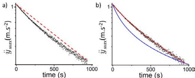
FIG. 7. (Color online) a) Maximum of the absolute value of the acceleration for each half period (black dots, in log scale). Exponential decay, as predicted by the damped harmonic oscillator model, would produce a linearly decreasing amplitude (red dashed line) which is obviously not the case. b) Numerical simulations: aerodynamic drag only (blue line) does not fit the data which is quite well reproduced by an almost equal contribution of viscous and aerodynamic damping (red line).
