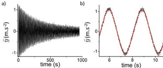
FIG. 2. (Color online) a) Raw data b) first few seconds of the record showing oversampling of the data allowing strong noise reduction through low pass filtering (red line).
