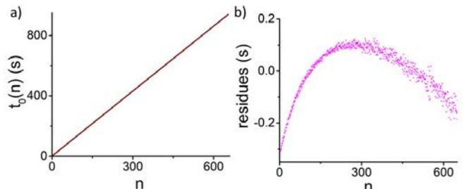
FIG. 5. (Color online) a)  $t_0(n)$  are the zero-crossing times of  $\ddot{y}$  successively numbered by  $n$  (black points). Red line: linear adjustment hardly distinguished from data points. b) Residual plot showing a significant departure of the oscillations from isochronism.
