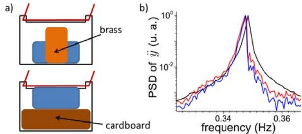
FIG. 3. (Color online) a) A piece of brass or cardboard is inserted in the envelope to change the total mass and mass geometry. b) Close view of the fundamental peak of FFT power density spectrum of  $\ddot{y}$ : smartphone alone (black), smartphone and brass piece (red), smartphone lifted up by a cardboard piece (blue). The slight decrease in frequency, is attributed to wires elongation after the heavy brass piece has been inserted.
